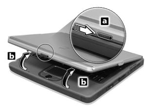
2 Push the display screen in the direction as shown in the illustration below until the "TIPS" stands firmly.
